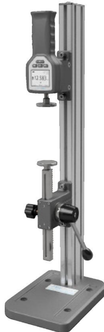
Shown: MTL-330 force tester with Metlogix DFG digital force gauge
