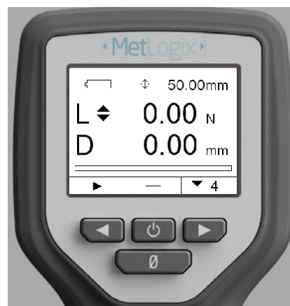
Shown: DFC Series displays both Load and Distance when connected to the FMM test frame.
